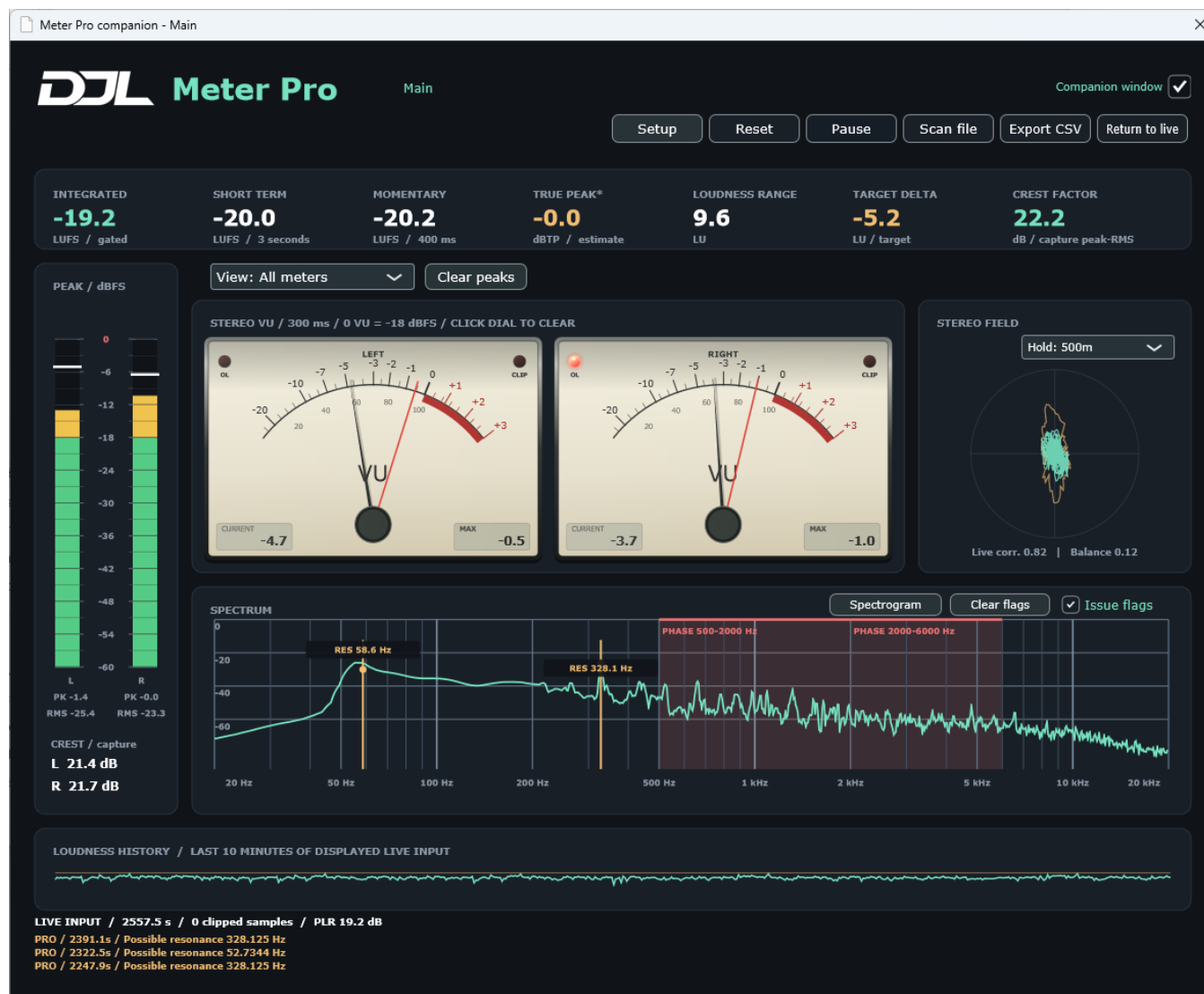
Figure 1. All meters in Meter Pro. Other editions show a subset of these controls and readouts.
